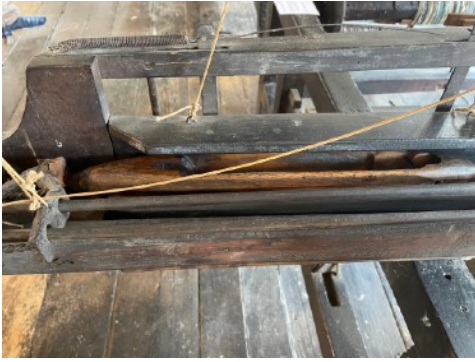
The Flying Shuttle in its shuttle box, ready to be thrown across the warp, using the pull strings
